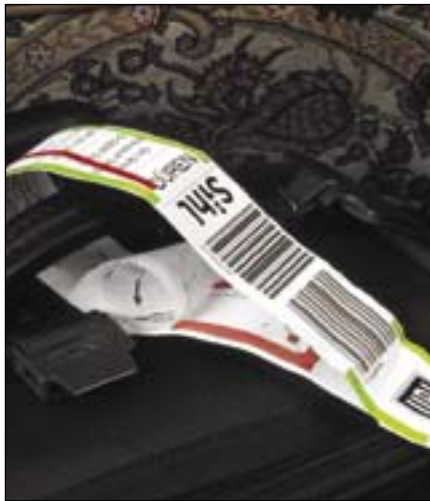
Above: A typical luggage tag with the RFID aerial seen as the copper coloured strip
