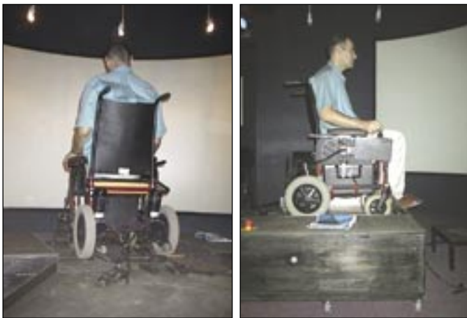
A motion platform is used to map wheelchair travel in the virtual world.
