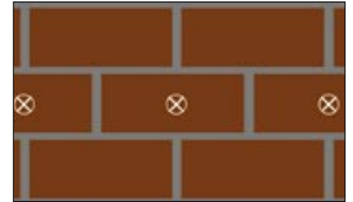
The Anti-Damp-Nozzle-Nub™ inserts, which are 22mm (nominal diameter) by 85mm long, are placed in the holes drilled into the bricks.
